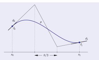
As illustrated in the figure, the Bernstein coefficients of the interpolant p form a polygon with equally spaced abscissae which touches p or, equivalently, the interpolated function at the interval endpoints. If Hermite data are given at more than two points, the cubic interpolants form a so-called Hermite spline q. By construction, q is uniquely determined by its values and derivatives at the interpolation points and continuously differentiable there.
