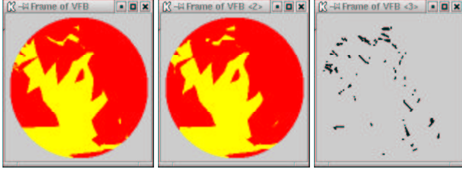
Figure 6: Left: the exact region R_p ; Middle: the approximate region R'_p computed by the radar-like algorithm; Right: \mathbf{XOR}(R'_p, R_p) .
