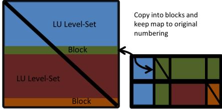
Figure 3: Level-set and block structure of **HiLUK**. Rows in level-set are kept in original order. Rows in blocks are copied to subblock structure with a map to original numbering.
