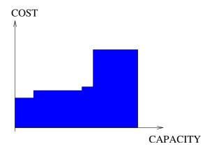
→ The cost of procuring capacity on a given arc is a step function – the function depends on the arc
