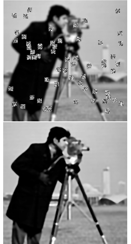
Figure 1. Bounded variation inpainting. Top, a blurry image with 60 packets randomly lost during the transmission process; bottom, after deblurring and error concealment by TV inpainting.
