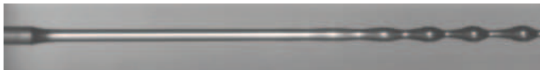
FIG. 1: A viscous flow down the outside of a thin vertical fiber; the surrounding fluid is air. The figure has been rotated by 90^\circ with gravity acting toward the right. Perturbations develop along the free surface some distance from the fluid source. Once formed, these perturbations continue to travel down the fiber. Image length is 9.7 cm.
