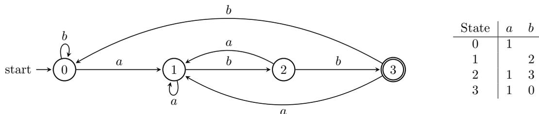
Figure 3: DFA transition diagram (left) and table (right) for the regular expression  $(a|b)^*abb$ .
