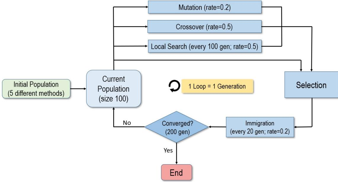
Figure 1: This flowchart illustrates the overall structure of our GA.
