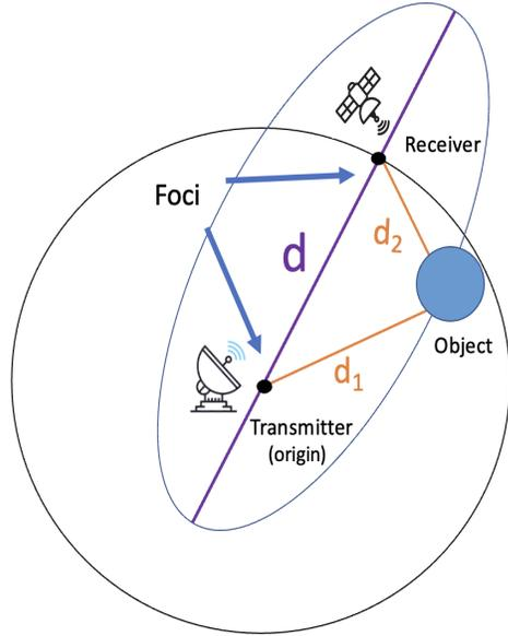
Fig. 1: Labeled bistatic radar system
