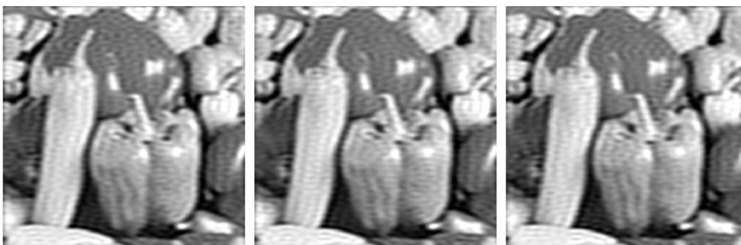
**Figure 14.** The restoration of a blurred image in the testing set with  $N = 512$ , using  $k_{GCV}$  as given in Table 3 for *gaussian*, *poisson* and *salt & pepper* noise, left to right plots respectively, and asymmetric blur. The relative errors for these images are all 0.118 with the same rounding as in Table 3.
