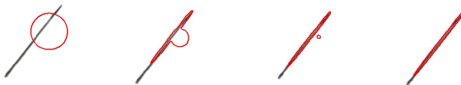
Figure 3: Locating a needle with the Chan-Vese algorithm.
