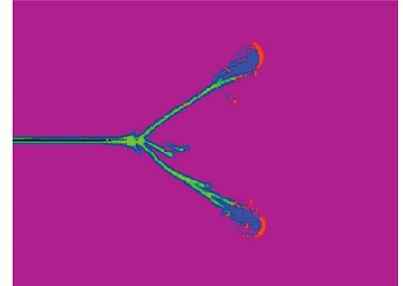
**Figure 1.** Peridynamic simulation of dynamic fracture starting from a short edge crack. Areas where damage has occurred are shown in blue and green. The active process zones where damage is increasing are shown in red. Because the plate is stretched at a constant rate, the cracks see a higher and higher strain field ahead of them as they grow.
