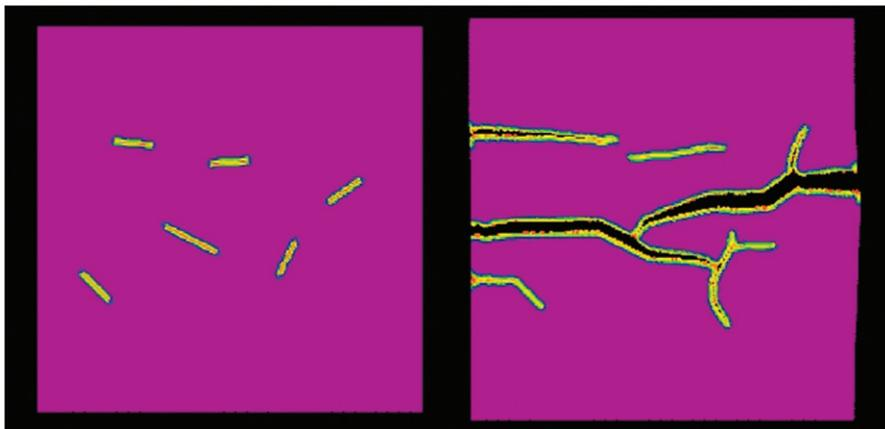
**Figure 2.** Simulation of the interaction of defects in a brittle plate stretched at a constant rate in the vertical direction. Left: initial defects. Right: growth and merging of defects, leading to macroscopic failure.
