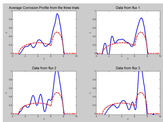
Figure 16: Reconstruction of large corrosion profile with k_2 = 0.1 , \alpha_2 = 0.2 .
